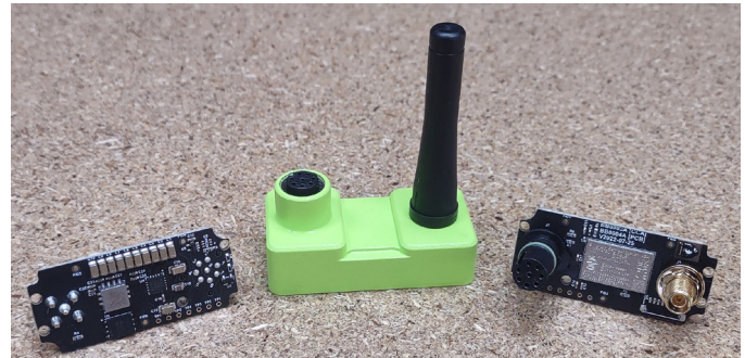
FIGURE 1. THE MACHINEMAILBOX : AN ACOUSTIC MACHINE MONITORING SENSOR USING THE NORDIC NRF9160 AND ZEPHYR.
